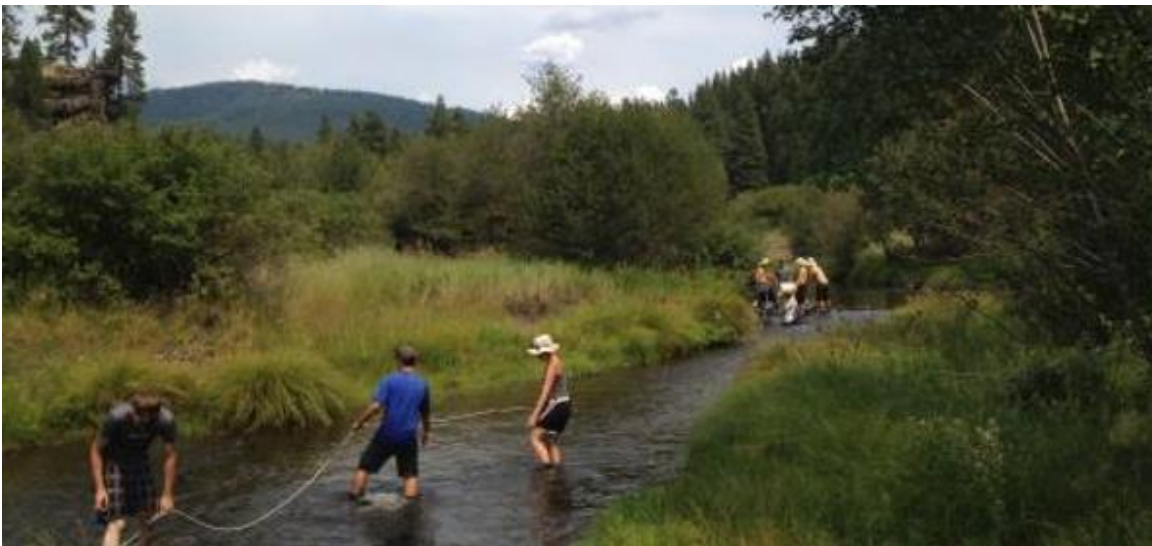
Figure 74 - Deploying a fiber-optic distributed-temperature sensor cable in the John Day River, Oregon, USA (OSU, 2020).
